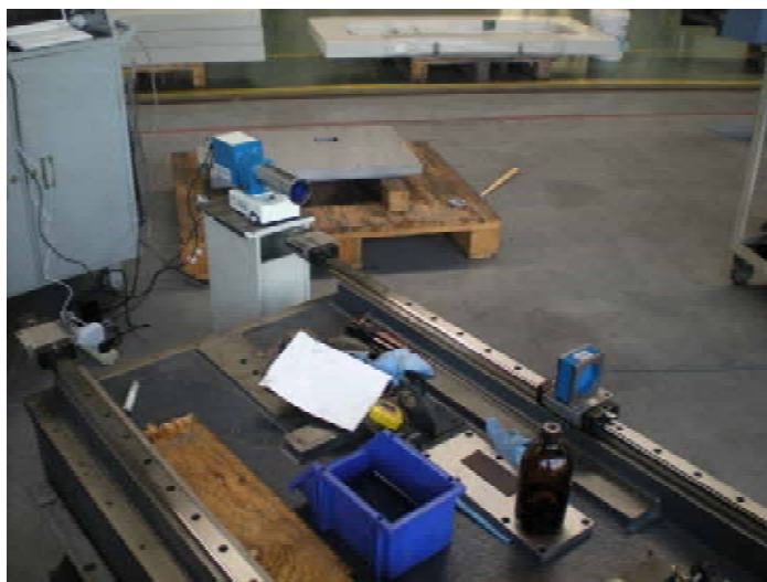
AutoMAT产品在现场测量加工中心导轨直线度 (Testing for straightness in the field)
